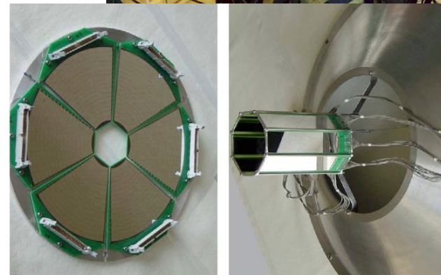
Left: Segmented backward annular detector (HYBALL). Right: Barrel.
